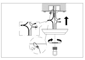
2. Connect the 3 power wires. The slick wires. The slick wire is the live wire, the coarse wire is the neutral wire, brass is the earth wire. Connect the wire lock.
