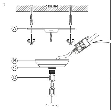
Turn off the electricity supply at the main circuit panel before installing. Do not connect the electricity supply until your luminaire is fully assembled and installed.
