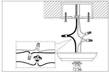
4. Loosen the retaining nut and move the canopy down. Connect the 3 wires. The slick wire is the live wire, the coarse wire is the neutral wire, brass is the earth wire. Slide the canopy up and fix it with the retaining nut.
