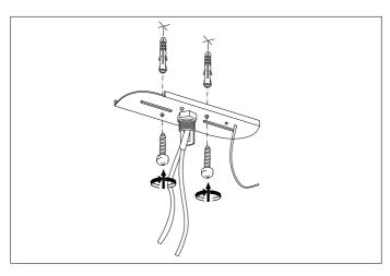
1. Lead the wires from your ceiling through the hole of the ceiling plate. Fix the ceiling plate to the ceiling by using mounting plugs and screws suitable to your ceiling type.
