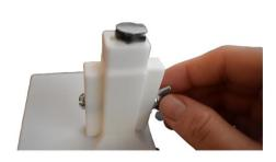
4) Continue feeding the zipper slider and pull tab into the top of the vice until it lays down flat. Once flat, tighten the zipper pull tab in place by turning the wingnut clockwise.
