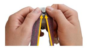
5) Begin to feed the zipper teeth upside down into the slider from either side of the slider. Take care to feed in the zipper teeth evenly on both sides. Feed the zipper tape in at a slight angle and it should slide inside the pull with relative ease.
