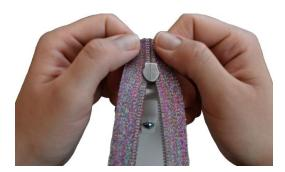
6) Continue to feed the zipper teeth fabric through the slider until a few inches of the zipper are closed on one side.
