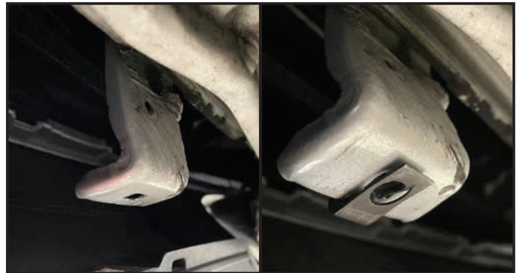
STEP 3 - METAL BRACKET BEFORE/AFTER CLIP-ON NUT INSTALLED
