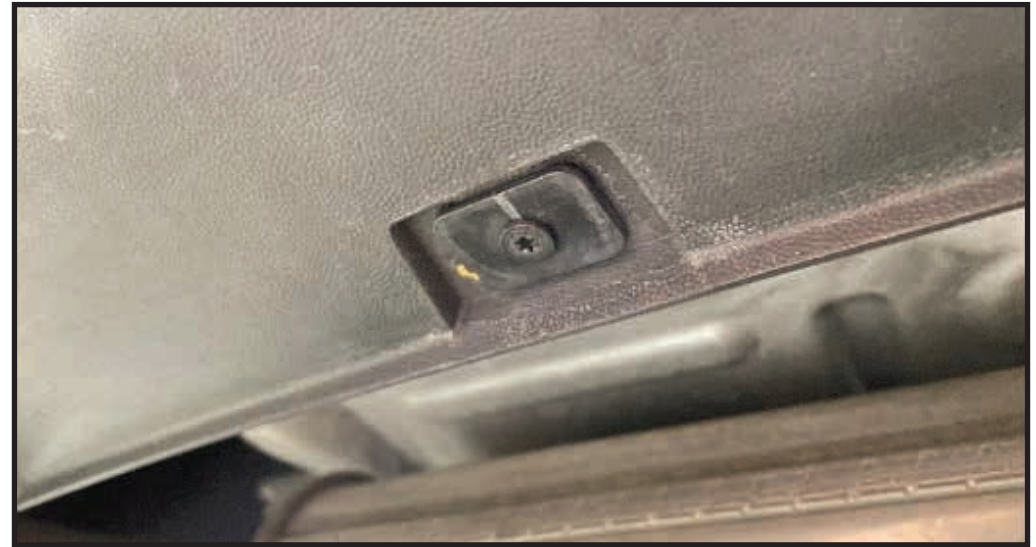
STEP 1 - PLASTIC SCREW UNDER OEM VALANCE
