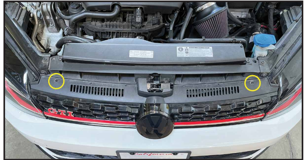
STEP 1 - UPPER GRILL BEFORE REMOVAL
