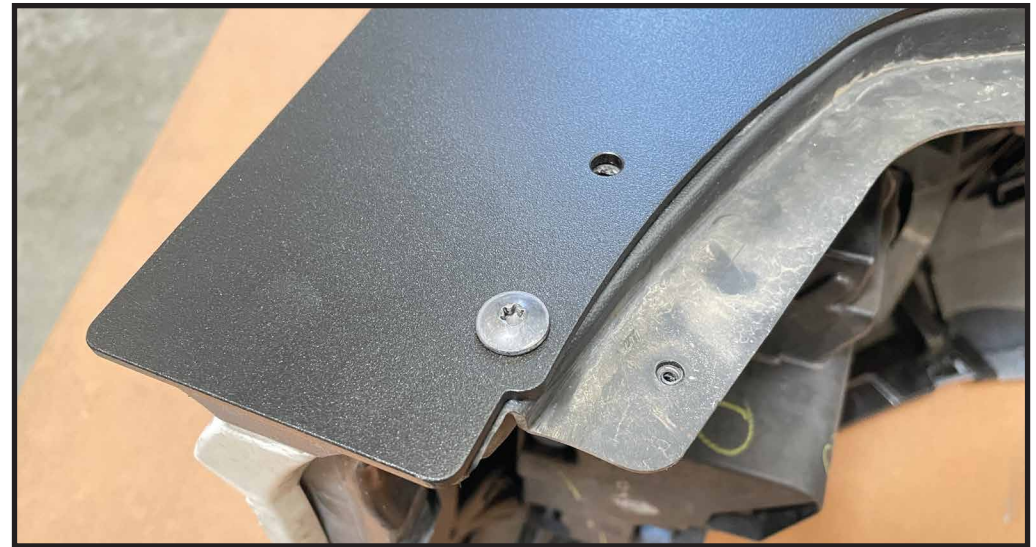
STEP 6 - TORX SCREW INSTALLED IN PRE-EXISTING HOLE
