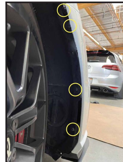
STEP 2 - FENDER LINER SCREWS
