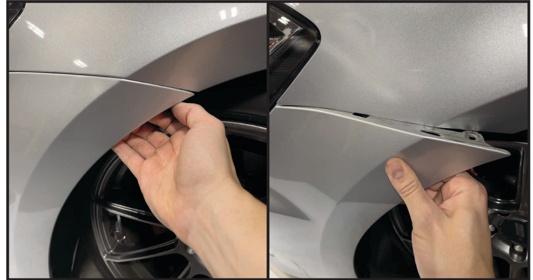
STEP 4 - PULLING FRONT BUMPER AWAY FROM CAR
