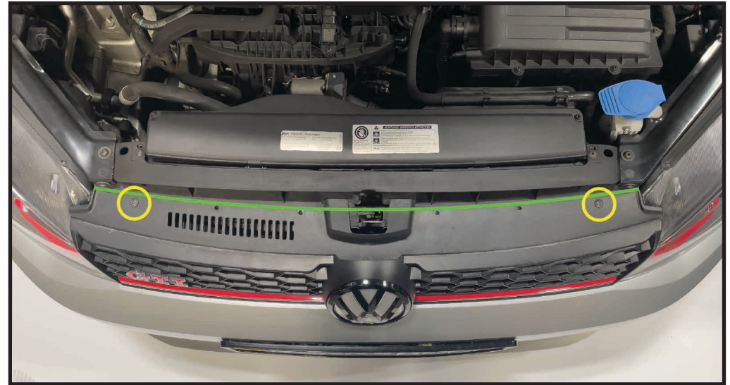
STEP 1.1 - UPPER GRILL BEFORE REMOVAL
