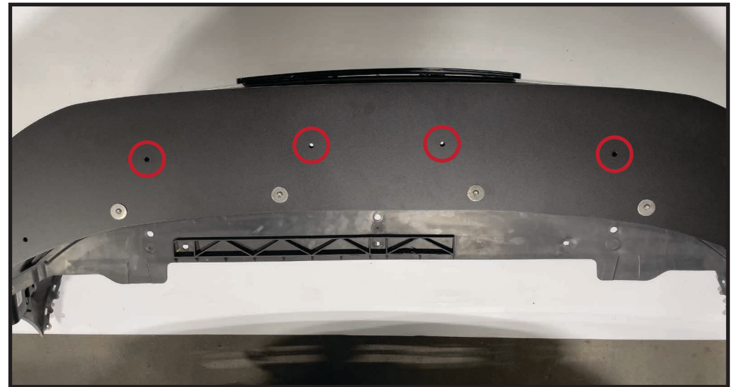
STEP 6 - BOLTS PLACED TO HELP ALIGN FRONT SPLITTER, DRILL HOLES CIRCLED IN RED
