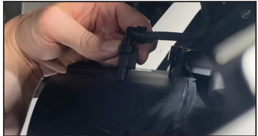
STEP 5 - DISCONNECTING FOG LIGHT
