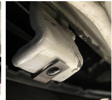
STEP 3 CLIP-ON NUT INSTALLED
