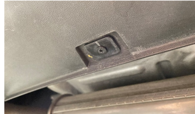
STEP 1 PLASTIC SCREW AND RETAINER UNDERNEATH OEM VALANCE
