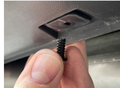
STEP 1 PLASTIC SCREW REMOVED
