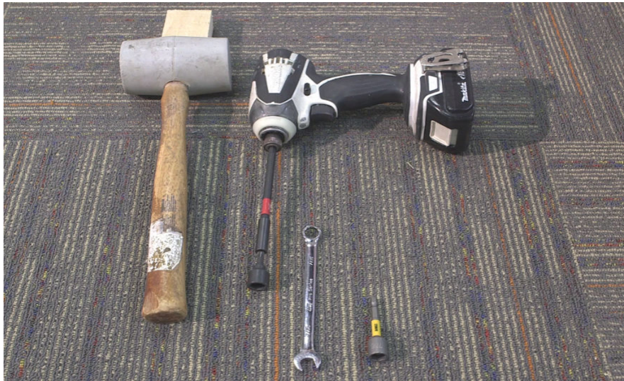
Tools: 1/2" & 7/16" sockets, 7/16" wrench, wood block 5" tall, or mallet plus wood block = 5" (Impact driver optional)
