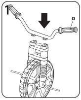
Turn the assembled front wheel upright. Place the handlebar (part O) onto the top of the front fork legs - in the groove between the screw holes.
