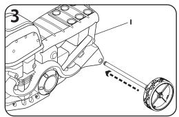
Slide the training wheel assembly into the Street Burner body (part I).
