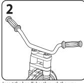
Insert the handlebar through the way down to screw compartment.
