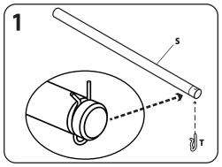
Install (1) locking pin (part T) into one end of the training wheel axle (part S) as shown.
