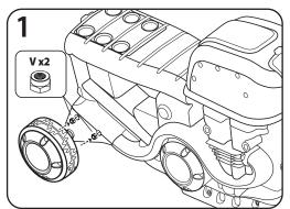
Locate the (2) hexagon nut holes. Insert (1) hexagon nut (part V) into each hole.
