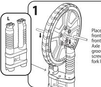
Place the assembled front wheel onto the front fork (part L).
