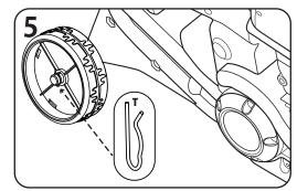
Install (1) locking pin (part T) into end of the training wheel axle (part S) as shown.
