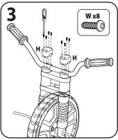
Place (1 each side) front fork - top (part H) over the handlebar. Secure the Front fork - top using (4) screws (part W) for each side. Tighten with screwdriver (included).
