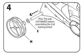
Slide onto open end of training wheel axle, (1) training wheel bushing (part E) then (1) training wheel (part M).
