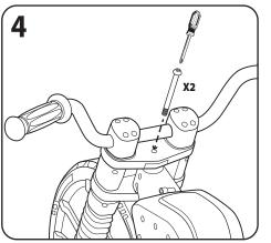
Insert (1) bolt (part X2) through the front fork assembly, through the front of the rear assembly, then into the hexagon nut in position under the front fork. Tighten with screwdriver (included). NOTE: be sure to hold the hexagon nut in place while tightening bolt.
