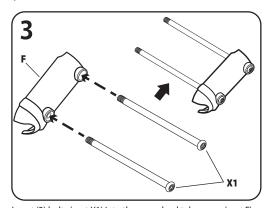
Insert (2) bolts (part X1) into the rear wheel tube cover (part F).
