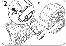
Insert the rear wheel assembly (part K) into the opening located on the opposite side of the Street Burner.
