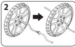
Insert the assembled front wheel axle through the front wheel (part J). Press the front wheel inserts into the center hub of the wheel. Inserts should be tightly fitted in center.
