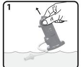
Fill with water: Submerge the hose tip under water and pull the top of the hydrant to fill it with water.
