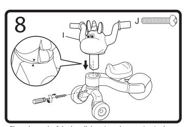
Place the neck of the handlebars into the opening in the center unit and align the arrows. Then, press down until it snaps into place. Using a Philip screwdriver (not included) install the screw (J) in the opening on the front of the wheel assembly.
