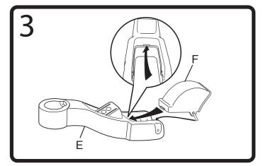
Place the pegs on the fender (F) into the slots on the fork of the center unit (E) and press them into place. Then, press down on the front edge of the fender until the lip of the fender snaps into the slot in the center unit.
