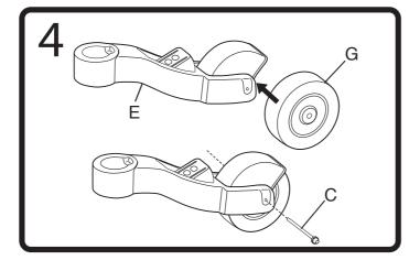
Place the back wheel (G) into the fork of the center unit (E). Slide the axle (C) through opening on the fender, wheel, fork assembly and out the other side.
