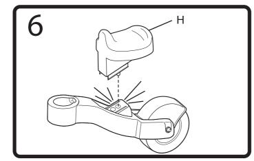
Place the seat onto the center unit, making sure the peg on the underside of the seat fits in the opening closest to the front of the rider. Press firmly until the seat snaps in place.
