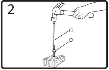
Place one axle cap (D), color side down, onto a piece of scrap wood (not included). Using a hammer, tap the axle (C) firmly onto the axle cap. Then, set it aside. Always wear safety glasses when using a hammer.
