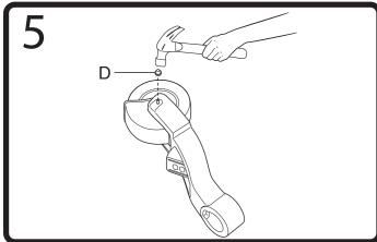
axle cap (D) onto the other end of the axle.
