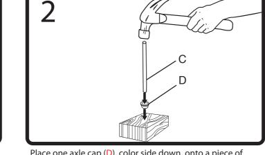
Place one axle cap (D), color side down, onto a piece of scrap wood (not included). Using a hammer, tap the axle (C) firmly onto the axle cap. Then, set it aside. Always wear safety glasses when using a hammer.
