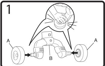
Place a front wheel (A) onto the peg on the front wheel assembly (B), making sure the word "inward" on the wheel faces toward the center of the unit. Press firmly until the wheel snaps in place. Repeat for the other wheel.
