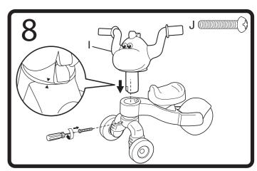
Place the neck of the handlebars into the opening in the center unit and align the arrows. Then, press down until it snaps into place. Using a Philip screwdriver (not included)
