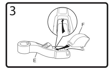
Place the pegs on the fender (F) into the slots on the fork of the center unit (E) and press them into place. Then, press down on the front edge of the fender until the lip of the fender snaps into the slot in the center unit.
