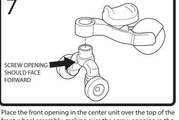
install the screw (J) in the opening on the front of the wheel assembly.
