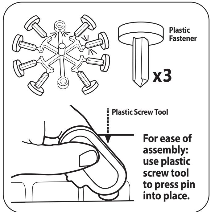
Break off a plastic fastener (x3) (spacer is NOT NEEDED). Insert the fastener (x3) in locations shown.
