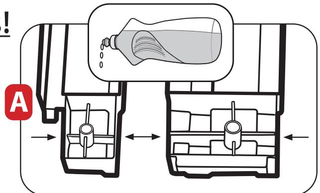
For Ease of Assembly: apply 1 tbsp. of liquid soap to surfaces of Wall Top (part A).
