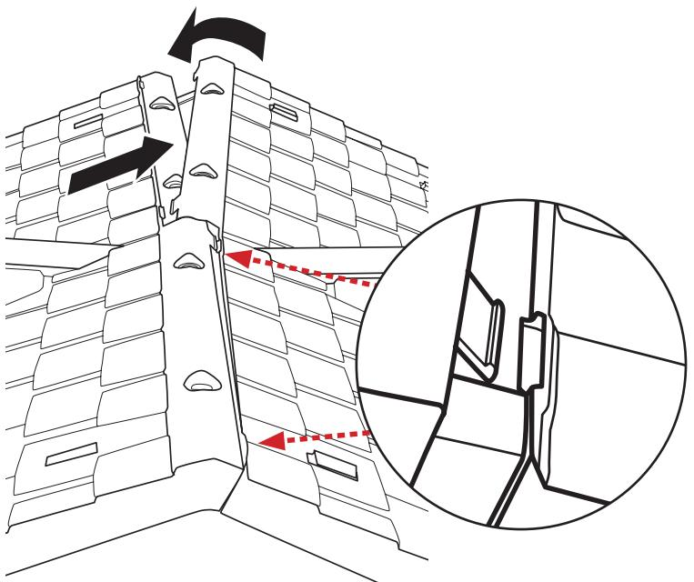
At the center of the roof, fit half of the roof peak
