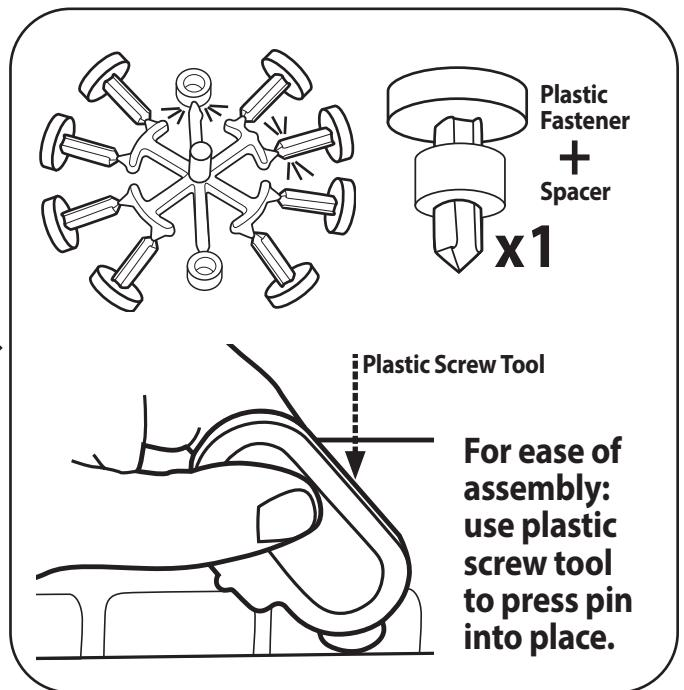
Break off a plastic fastener and spacer from ring. Place spacer onto the fastener and insert it into the hole located on the raised brick as shown.
