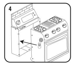
Slide the front of the oven into the back wall, making sure the openings on the sides and the one on the bottom align.
