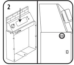
Insert the top panel on top of the back wall of the oven. The openings on each side should align.
