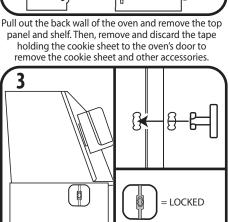
Insert a screw on each side of the top panel and turn the screw to lock in place. The screw should enter both openings.
