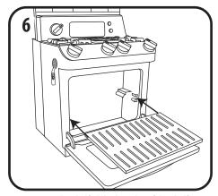
To insert the shelf, slide the sides of the shelf in between the brackets in the oven.
