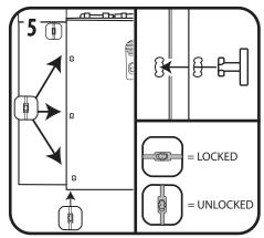
Insert three screws on each side and one screw on the bottom. Make sure the screw enters both openings. Then, turn the screw to lock in place.
