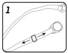
Adjust the bandolier by pulling up or down the clip on the strap. Adjust so it fits comfortably on your body. Do not over-tighten.
