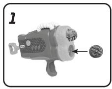
Holding the blaster in an upright position, insert the power pods.
