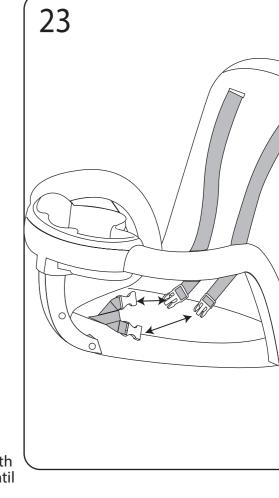
To adjust the center seat belt length, follow the path shown above. Pull seat belt tail through the clip until it is tight and secure.
