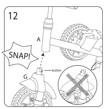
Press frame (A) and front wheel (G) together until the button snaps into place.
