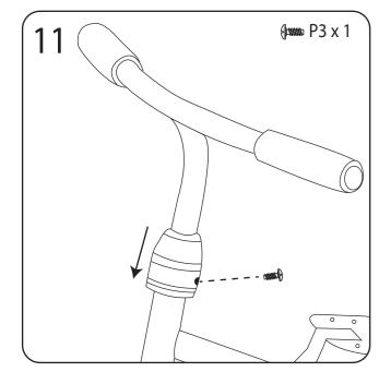
Push cap (E) down and secure with a screw (P3).
