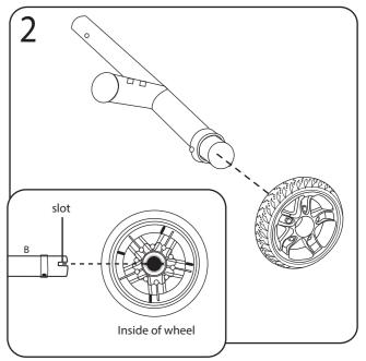
Align slots on wheel center with slots on axle (C).
