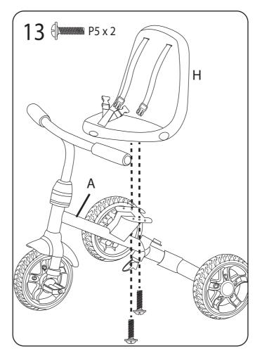
Insert screws into the same openings on both sides of the seat.
