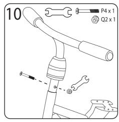
Place washer over the frame (A). Then, completely push the handlebars down.
