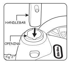
2. Place end of the scooter handlebar over the body opening. (Fig. 2)
