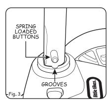
3. Slide the end of the handlebar into the opening making sure the spring loaded buttons on both sides of the handlebar fit into the grooves in the opening. (Fig. 3)
