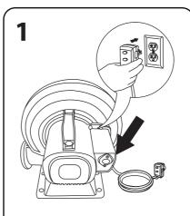
Switch power ON. If blower does not operate when switched on, press the reset button on the GFCI adapter.
