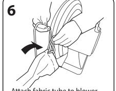
Attach fabric tube to blower unit making sure the tube is not twisted.
