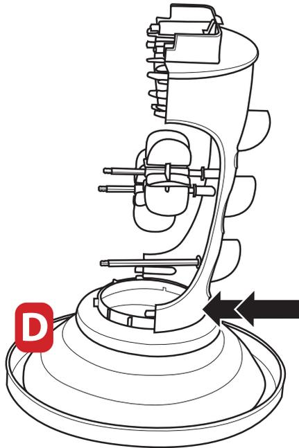
Align tower connector rods to the holes in the tower RIGHT.
