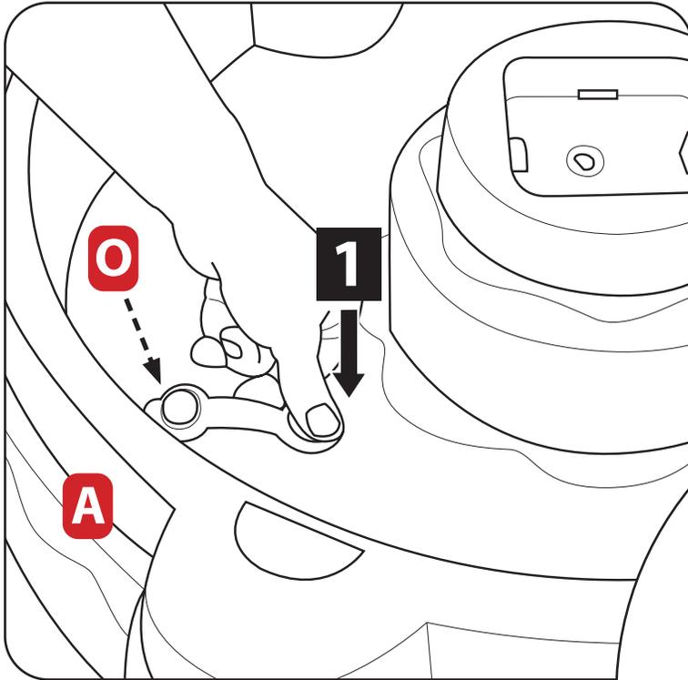
Next, flip table over. Work the plug around the opening, pulling only the plug edge through.
