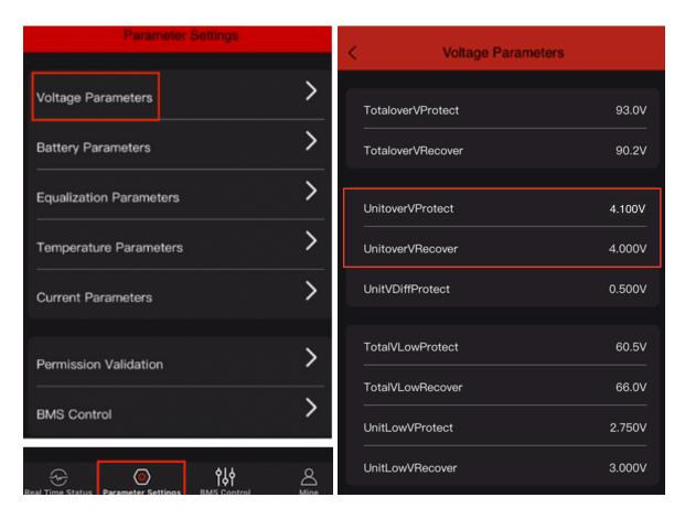
In the Parameter Settings menu, change: UnitoverVProtect to 4.1v and UnitoverVRecover to 4.0v
