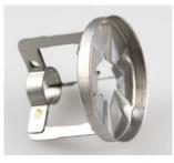
AIR NOZZLE If the air nozzle is extremely sooty, the burner has been affected by a lack of ventilation and it requires changing. AH10028
