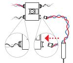
Remove the drone's bottom chassis. Then check if the motor is disconnected from the drone's board.
