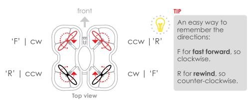
Please note, a **propeller's color does not indicate its rotation**. However, we recommend placing the red propellers at the front of the drone. This will help identify the front of the drone during flight.
