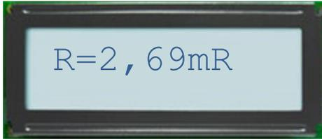
The displayed value is the measured ohmic resistance (milli-Ohms) of the entire electrode system. The internally stored calibration is now updated with the new results.
