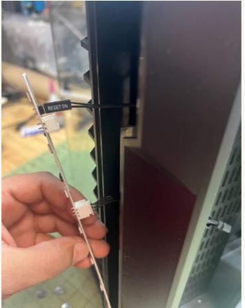
Carefully pull the LED strip away from the case to remove.
