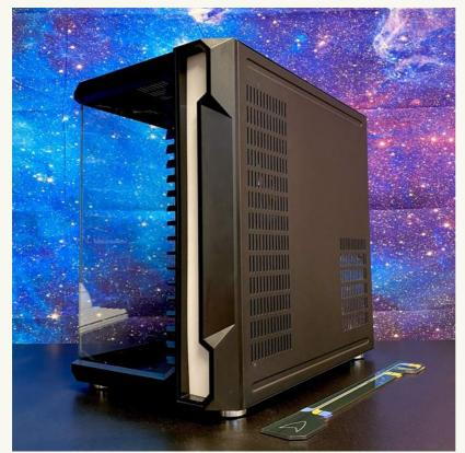
The faceplate sits in front of the white diffuser plate, on the front panel of the case.
