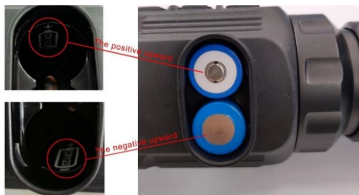
Fig. 8-1 Schematic diagram of battery installation
