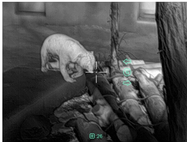
Fig. 6-3 Blind pixel correction interface
