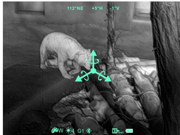
Fig. 6-5 Compass calibration interface
