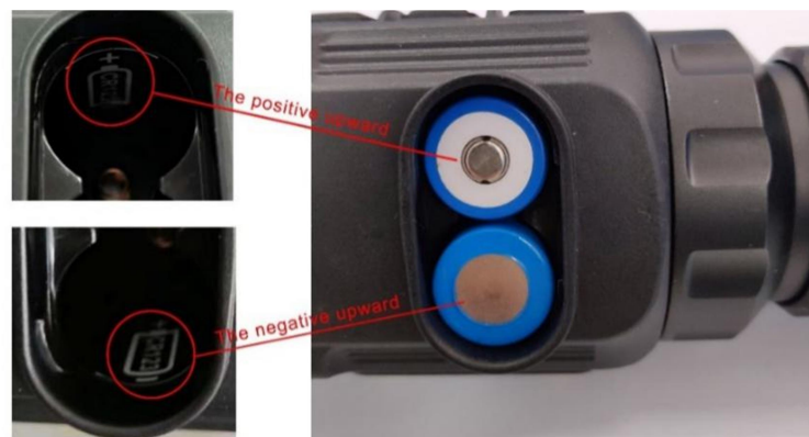
Fig. 8-1 Schematic diagram of battery installation
