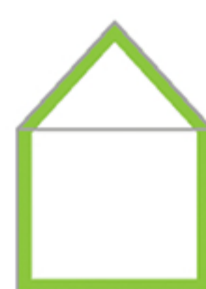
Optimal interior insulation
