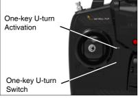
instead of to the transmitter, which means the plane will U-turn ONLY to the opposite direction that the plane takes off. It also means when the plane U-turns and passes the position where you activated the function, the one-key U-turn function will NOT U-turn the plane back to the take-off position.
