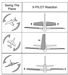
Place your plane in a neutral position, follow below steps to check the channels reactions. Move the sticks(except the throttle stick) to see if all servo surfaces react correctly as shown in the left diagram(left throttle for example). Swing your plane to check if all servo surfaces react correctly as shown in the right diagram.
