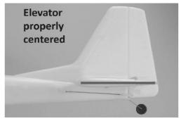
Then observe the elevator to ensure it is properly centered as shown above.
