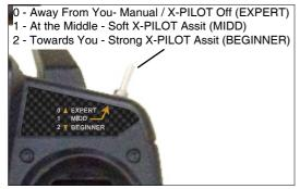
The airplane comes with pre-installed X-PILOT to help control flying easily. The switch is with 3 levels to control the X-PILOT. To turn on the X-PILOT, switch to upper position(towards you). To turn off the X-PILOT, switch to lower position(away from you).
