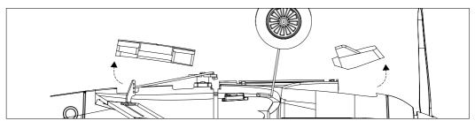
1. Take off the cover in the head of fuselage to replace the motor, or the cover in the middle of fuselage to replace the receiver. It is no need of tool to take off the covers.
