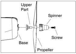
Follow below steps to replace broken propeller and shaft adaptor. You will need help of a Philips screw driver and pliers(not included).
