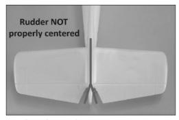
Observe the rudder to ensure it is properly centered as shown above.
