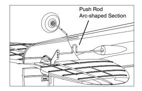
If the elevator is angled off to the upper or lower position, adjust the push rod by its arc-shaped section slightly, making sure the elevator is properly centered.
