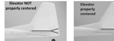
Then observe the elevator to ensure it is properly centered as shown below.
