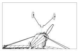
2. Plug the landing gear into the fuselage as shown above.
