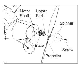
The propeller saver keeps the propeller from damage, and prevent the electronic components from over current. When the airplane hits any obstacle, the propeller will loose from the base. To install the propeller back to the base, insert the upper part centerly through the motor shaft, and hearing a "click" sound to ensure it is secured.
