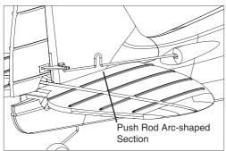
If the rudder is angled off to the right or left, adjust the push rod by its arc-shaped section slightly, making sure the rudder is properly centered.
