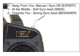
The Sport Cub S2 comes with pre-installed Gyro to help control flying easily. The switch is with 3 levels to control the Gyro. To turn on the Gyro, switch to upper position(towards you). To turn off the Gyro, switch to lower position(away from you).
