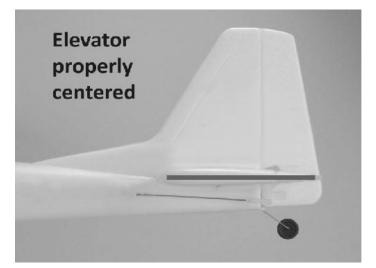
Also, we strongly recommend installing the included 'clevis keepers' to provide added security for the clevises. Typically you can carefully slide the keepers over the clevises when they are not connected to the control horn. Then, after connecting the clevis to the control horn and 'snapping' the clevis together you can slide the keepers into a position that does not allow them to 'bind' against the control horn during movement of the surface.
