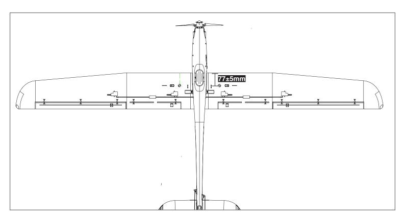
The ideal C.G.position is **77±5mm** behind the leading edge measured at where the wing meets the fuselage. The C.G. has a GREAT effect on the way of the model flight. If the C.G. is too far back (tail heavy), the model will be too responsive and difficult to control. If the C.G. is too far forward (nose heavy), the model will be too stable and not responsive enough. In order to obtain the C.G. specified, add weight to the fuselage or move the battery position. Check the C.G. before flying.
