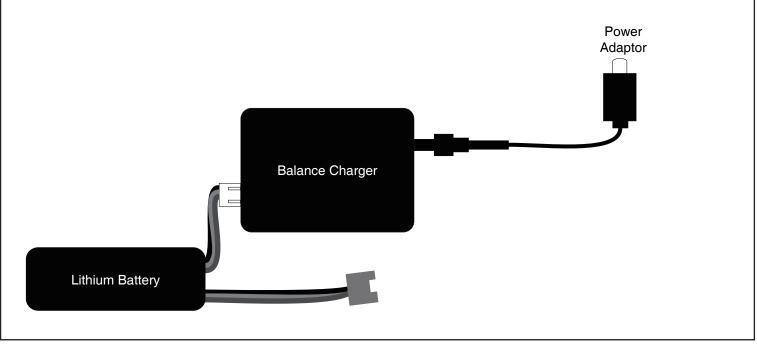
For charging the included lithium battery, you can only use the included charger set(balance charger and power supply), or a suitably compatible lithium battery charger.
