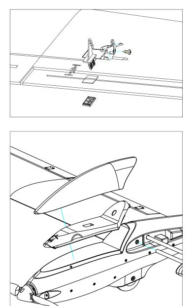
8. Depends on what feature you need, cover on the camera mount(for FPV flight) or the canopy(for normal flight).
