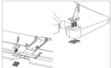
2. Install hinge control horns to reserved position on vertical tail and horizontal tail. Make sure it is well secured.
