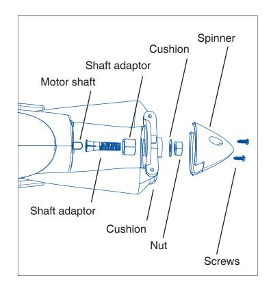
9. Install the propeller to the motor shaft by the order as above.
