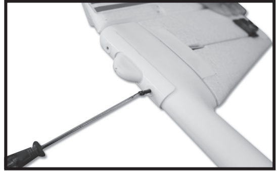
3. Connect the servo wire of the tail.
