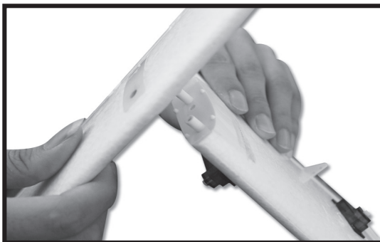
6. Install the elevator to the rudder by screw.
