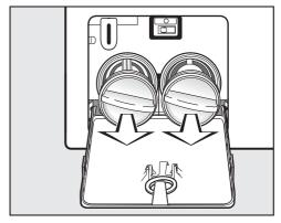
■ Remove the drain filters completely.
