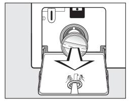
■ Remove the drain filter completely.
