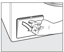
■ Open the drain pump access panel.
