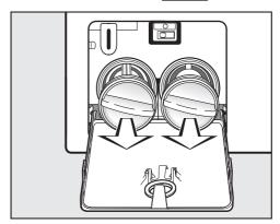
■ Remove the drain filters completely.
