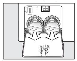
■ Remove the drain filters completely.
