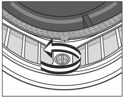
■ Turn the yellow dial on the lower fluff filter in the direction of the arrow (until it reaches the stop position).
