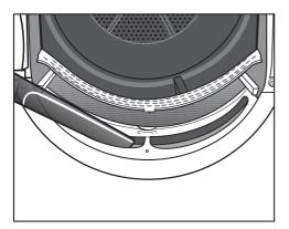
Use a vacuum cleaner with a long crevice nozzle attached to remove any visible fluff from the upper air flow openings.
