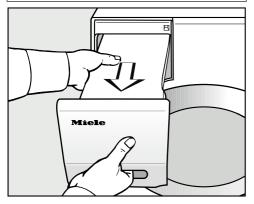
Remove the condensed water container.
