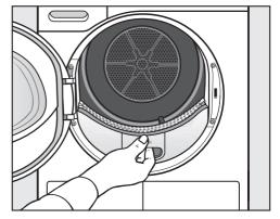
■ Pull the upper fluff filter forwards to remove it.
