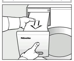
Remove the condensed water container.
