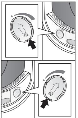
Open the cover using the tab until the tab is right at the top as shown.
