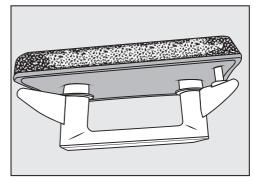
These residues arise from laundry fibres and traces of detergent components. They can be found on the front and side edges of the plinth filter. In extreme cases, they can form stubborn crust. Residues are a sign that the plinth filter no is longer a snug fit at the sides, even if it appears to be perfect: fluff is getting in unfiltered at the edges.
