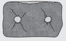
Fluff will blow into the heat exchanger through cracks and tears. This will, in time, cause a blockage in the heat exchanger. White residues or residues of other colours
