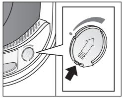
Push the tab down completely (see arrow) so that the socket is closed.
