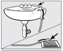
Should the end of the hose come loose, overflowing water can cause damage.
