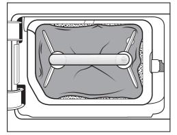
The edges of the plinth filter do not sit properly and the plinth filter is out of shape. Fluff will blow into the heat exchanger unfiltered through edges that do not sit properly. This will, in time, cause a blockage in the heat exchanger.
