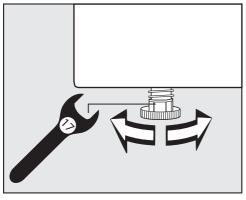
Turn the screw feet by hand or with a flat open spanner.
