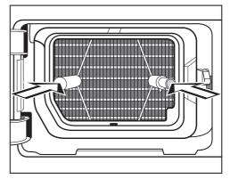
■ Push the plinth filter in completely.
