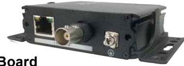
IPC Left Board EPOC, Grounding Terminal
