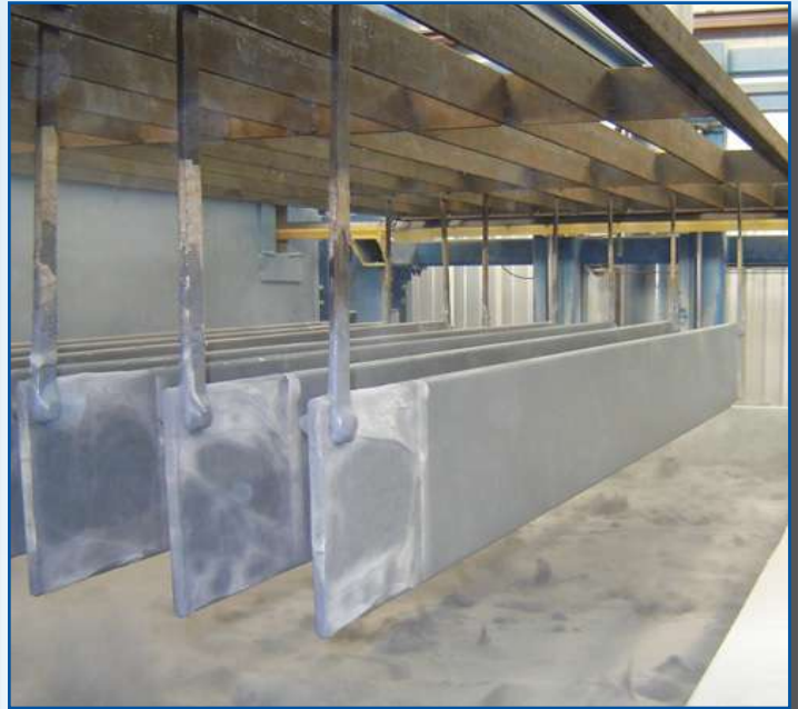
Epoxy Coating System
