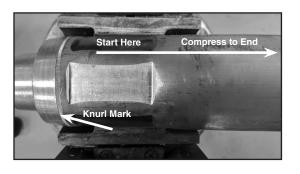
Step #9 Continue to compress until the compressions meet the inside of the knurl mark closest to the jumper pad.
