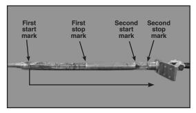
NOTE: If aluminum tube is touching the seal before reaching the First stop mark then stop compression and move to step #17.
