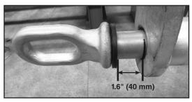
NOTE: This distance can vary  $\pm$  0.20" (5mm), installer may adjust after first compression is complete
