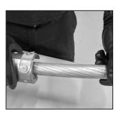
hardware (at least the length of the jumper inner aluminum sleeve) per your standard company practices. Check that no residue or surface particles remain.
