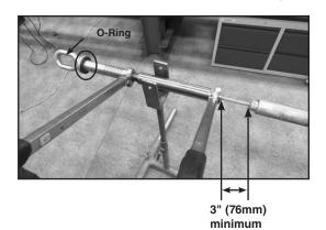
Step #13 Slide the aluminum outer sleeve towards the eye, lining up the edge of the pad with the mark on the steel eye. If no mark is present, offset the dead-end eye to dimension in table in step #1 column Eye Distance.
