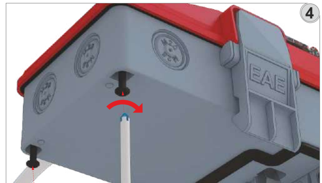
4- Tighten the removed cover screws.
