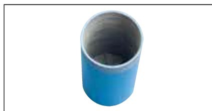
Fig. 13 The bottom of the tube contains compressed material (starting material). Tap the bottom of the tube a couple of times to loosen this material.
