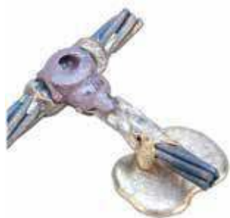
Reject. A worn or incorrect mold was used, allowing leakage around conductor. The fill in this connection is insufficient to allow it as acceptable. Replacement of mold is required prior to making next connection.
