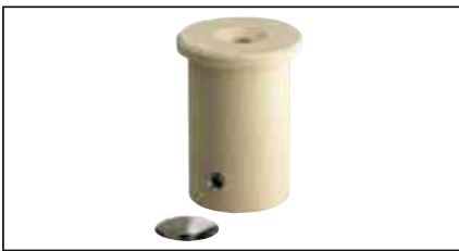
Fig. 3 Check to ensure the ceramic mold is not broken, which could cause leakage of molten weld metal during the reaction.
