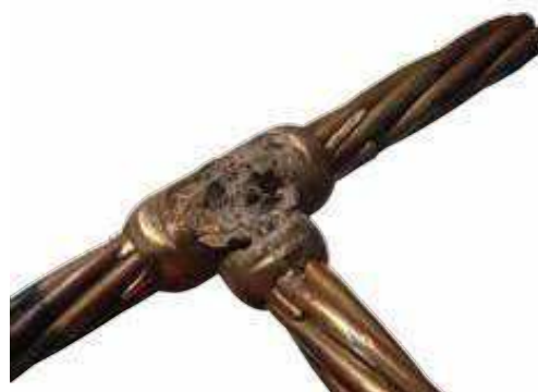
Reject. Fill too low. Weld cavity was not filled over cable strands. Absence of leakage indicates that welding material size was incorrect (too small) or thru conductor moved.
