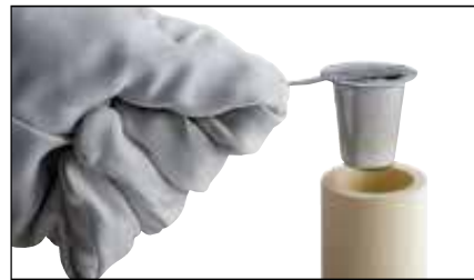
Fig. 9 Place the welding material cup into the top of the mold. Make sure the ignition strip nests into the recess on the top edge.
