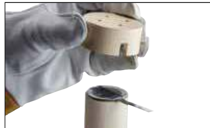
Fig. 10 Place the ceramic lid onto the mold.
