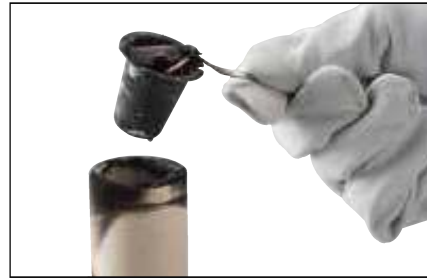
Fig. 14 Remove and dispose of the used Cadweld Plus weld metal cup.
