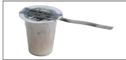
Fig. 8 Inspect the cup to ensure it is tightly sealed and the ignition strip is securely attached to the seal.
