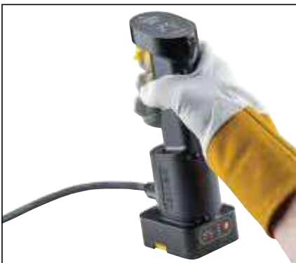
Fig. 13 Using the control unit, lift the trigger cover and press the ignition button and hold. You will see the 6 lights on the top of the control
