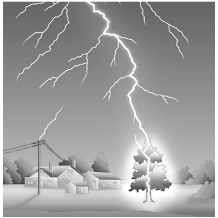
Figure 5. Upward leaders propagate toward downward leader to complete the ionized path between cloud and ground.
