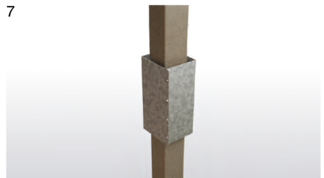
7 Gaskets must be located only bottom part of the mould plates. By this way resin can be poured from top side.
