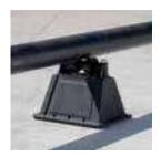
Material: Polyethylene, Polypropylene, Steel Finish: Hot-Dip Galvanized Temperature: -50 to 150 °F Static Load Safety Factor: 3:1
