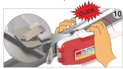
First, connect product earth terminal to busbar plug-in point. Then make sure that other terminals connect to busbar. Finally you should hear "CLICK" sound when you press tap-off box towards busbar.
