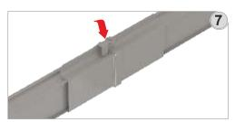
By closing the snap-in latch, you may complete the snap-in connection.
