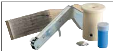
Fig. 2 Gather the proper materials and equipment for the type of connection you are making. The Cadweld One Shot system requires a Cadweld One Shot ceramic mold, welding material, wire brush for cleaning/preparing conductors, flint igniter, and propane torch.
