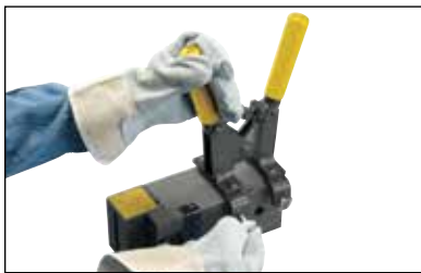
Fig. 7 Tighten the clamp thumbscrews onto the mold.
