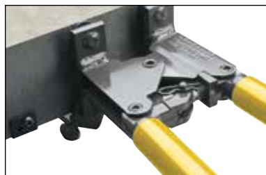
Fig. 9 If the mold does not seal properly, make adjustments to tighten/loosen the handle clamp.
