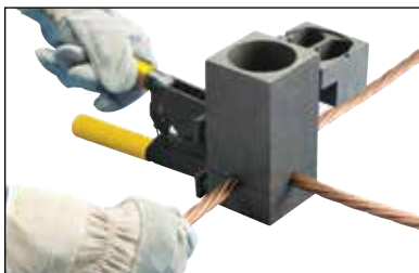
Fig. 13 Insert the conductors and position them for the connection.
