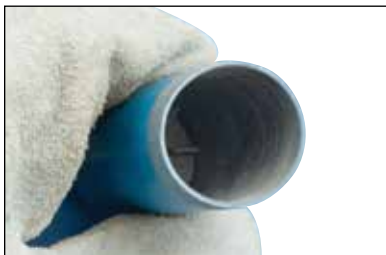
Fig. 21 The bottom of the tube contains compressed material (starting material). Tap the bottom of the tube a couple of times to loosen this material.
