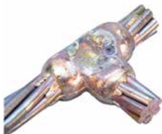
Acceptable. Fill is lower than normal, but still sufficient.
