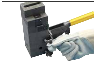
Fig. 7 Tighten the clamp thumbscrews onto the mold.
