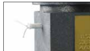
Fig. 23 Next, take an igniter pin and place it halfway into the small hole on the side of the mold, with the loop side facing into the hole. Spread the wire leads.
