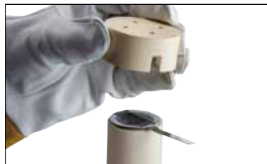
Fig. 10 Place the ceramic lid onto the mold.
