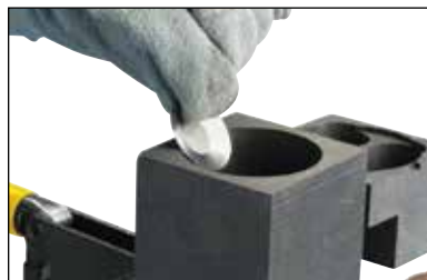
Fig. 16 Insert the steel disk (concave side up) into the mold. Hold the steel disk on the side of the mold and let it slide into place.
