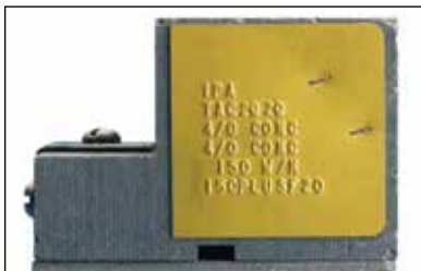
Fig. 4 Inspect the mold ID tag to ensure that it corresponds to the application, indicated by the:
