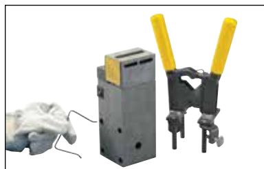
Fig. 5 Remove the small wire bracket which is used to temporarily hold the mold together before using. Set the bracket aside.
