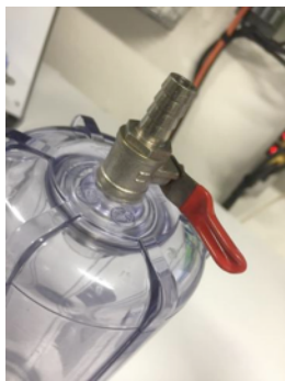
Valve installed (make sure that the lever opens the valve away from the filter when installing!)
