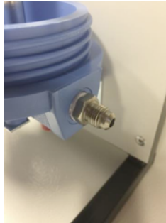
1/4" NPT Male to 1/4" MFL Adapter installed
