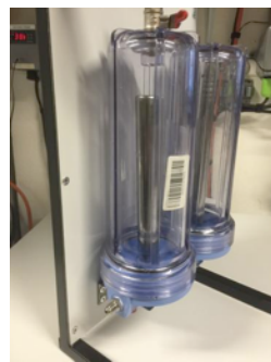
Valve installed at top (or bottom) of de-foaming chamber (L) View showing center tube length in de-foaming chamber (R)
