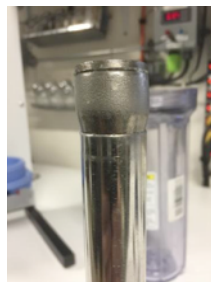
Tubing cutter, Tapered spear end and tool used to correct taper (L) Hammering this stainless reducer into the tubing corrected the taper issue (R)
