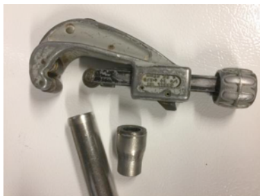
Tubing cutter, Tapered spear end and tool used to correct taper (L) Hammering this stainless reducer into the tubing corrected the taper issue (R)
