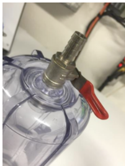
Valve installed at top (or bottom) of de-foaming chamber (L) View showing center tube length in de-foaming chamber (R)
